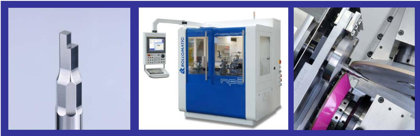
Pinch grinding offers highest concentricity particularly on long and thin parts. The rough and finish grinding are performed in one pass (patented). This innovative way to grind roughing and finishing simultaneously eliminates a separate process and reduces cycle time. The machine utilizes two different grinding wheels running on separate spindles and positioned on independently-controlled CNC linear slides.
